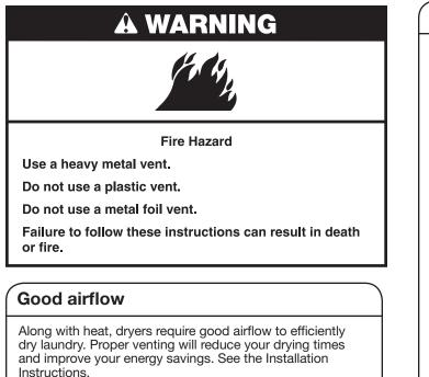
The venting system attached to the dryer plays a big role in good airflow. Blocked or crushed vents as well as improper venting installation will reduce airflow and dryer performance.
